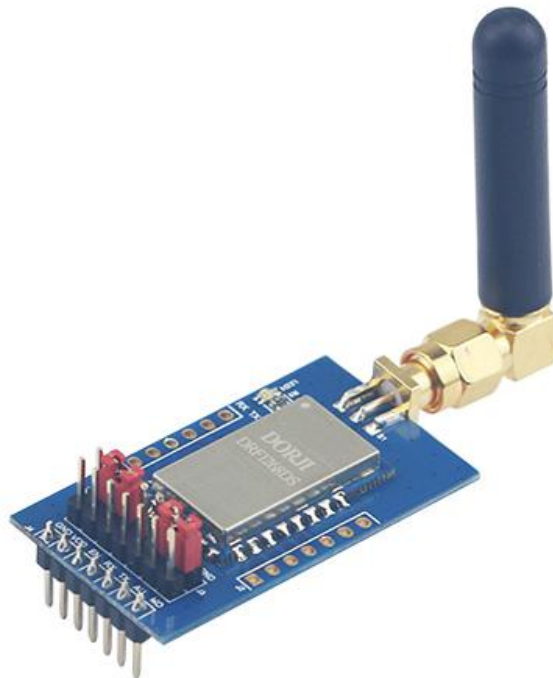
Figure 9: DAD07 Board with DRF126xDS Module Installed
